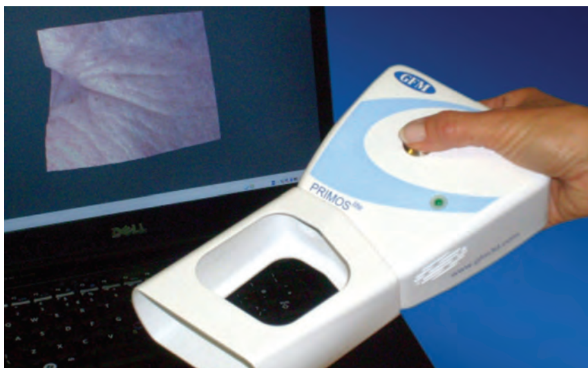
Figure 3 The Primos 3D device for assessment of the skin roughness and wrinkle reduction
